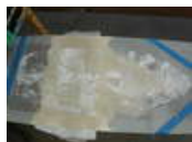
How to Fiberglass: Fixing a Cracked Kiteboard by noahw
